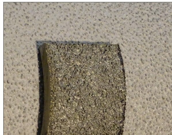
Figure 5. Spiny type as-cast surface (bottom) compared to rough-liner surface (top)
